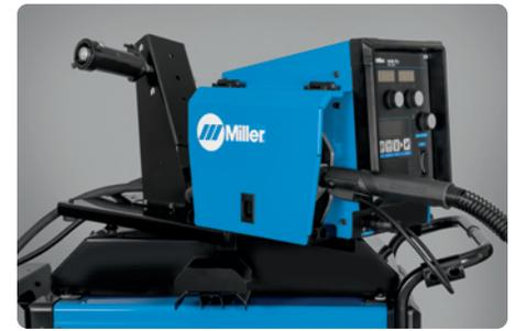
**Single-wire feeder swivels** for convenience and function, eliminating wear on gun and liner assembly. It moves with the MIG gun, allowing operator to see the front of the feeder and which parameters are selected.
