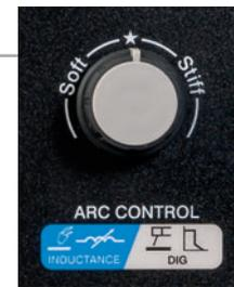
**Arc control** is active in the stick and solid-wire processes. It allows the operator to customize arc characteristics to match preference, electrode and joint design from a softer arc with more fluid puddle to a stiffer arc with an more controllable puddle. The Star setting is optimized for most applications and pointing the control at Soft or Stiff is optimal for most arc preferences. Control is fully adjustable from 0 to 25 Soft or 0 to 25 Stiff.
